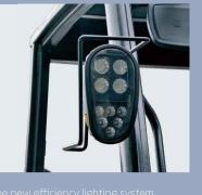
ne new efficiency lighting system nploys LED illuminant and new type flector to reduce energy consumption, prove significantly illumination erformance and prolong work time
