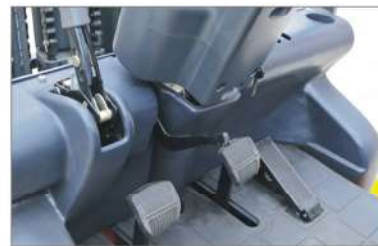
Cowl mounted hydraulic lever offers large operation space.
