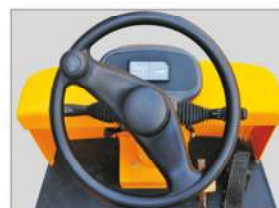
Adjustable steering column with electric F/R lever.
