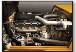
**ENGINE:** The M Series forklifts have a sliding hood for easy access during maintenace, and house a Perkins Turbo Tier 3 emissions compliant diesel engine.
