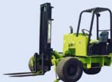
P Series Forklifts Capacity: 6,000 - 50,000 lb Straight Mast 4WD, 4WS
